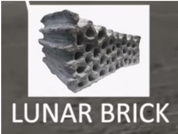
Below: A construction material synthesised in situ using lunar regolith.
